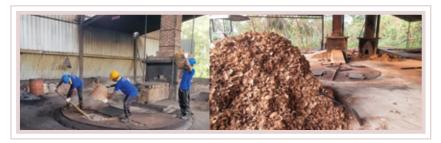
introducing closed-pit burning of coconut shells, drastically reducing air pollution and toxic gas emissions. As a result, 91% of Sri Lanka's charcoal is now produced using cleaner methods.
